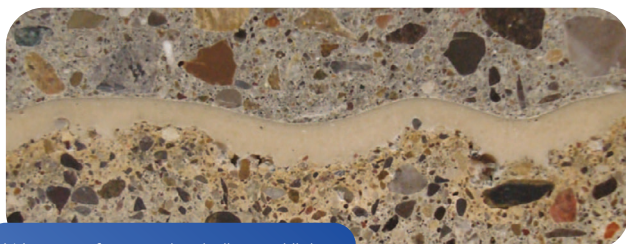
Waterproof composite shell tunnel lining
