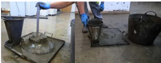
Figure 2. Without ad-mixture (left), and with MasterRoc MF (right).
